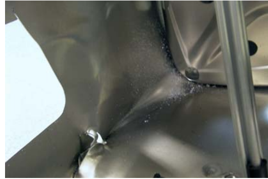
Fig. 2 Corrosion free inside of a 7 year old aluminium truck fuel tank
